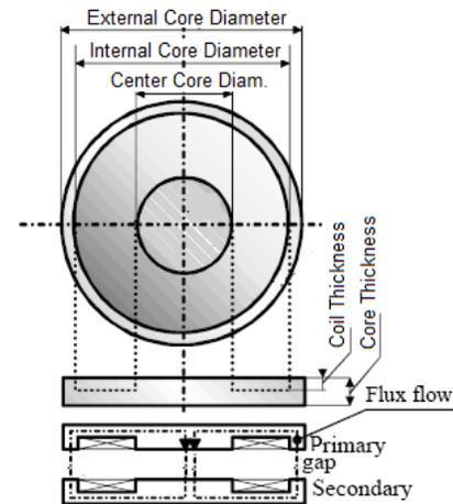
Fig. 2. Geometry of the considered transformer
