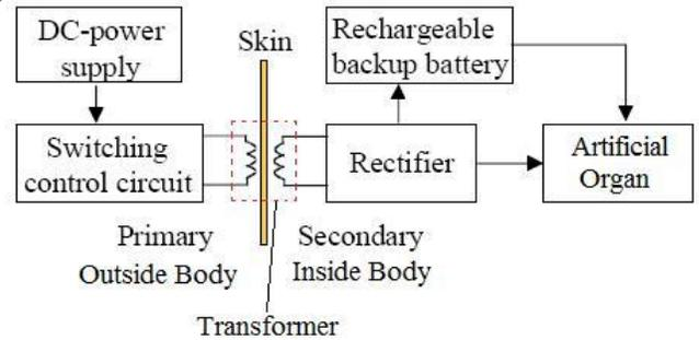
Fig. 1. Block Diagram of the considered TET
